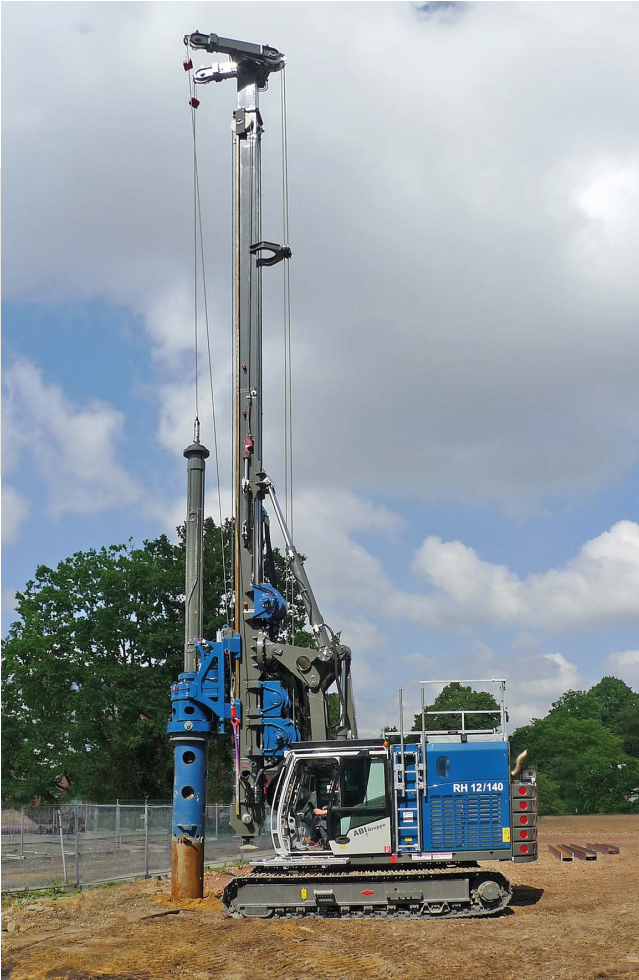
The smallest model of the DELMAG rotary drill rigs while Kelly drilling. The machine can be transported with the rotary head and Kelly bar still attached.
