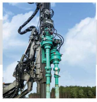
For soil mixing, productivity can be increased by using multiple auger drives.
