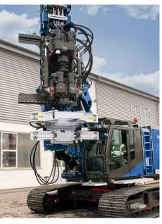
ABI MOBILRAM TM 17 with micro pile equipment, the auger drive can be moved lateraly out of the drilling axis, the clamping and breaking device is used for handling the single micro pile elements.
