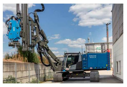
ABI MOBILRAM TM 20 LR- one machine with longer reach, primarily designed for working below or above the work platform, e. g. for pile driving elements on embankments, near roads or motorways.
