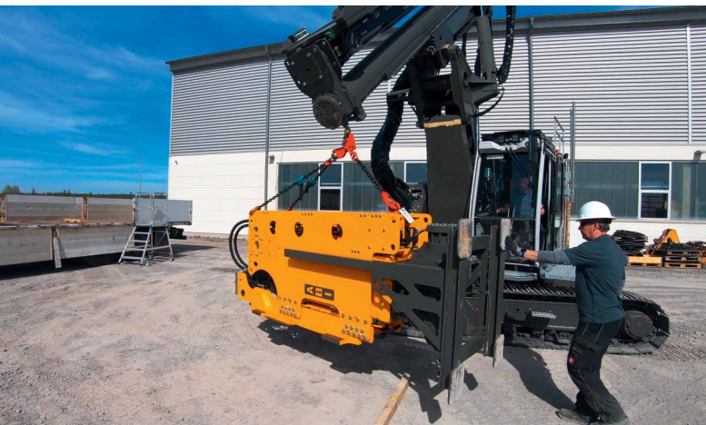
Photo: Job site of Dawson WAM Ltd - ABI MOBILRAM TM 13 with vibrator MRZV 12VV working on the smart motorway project (above)
