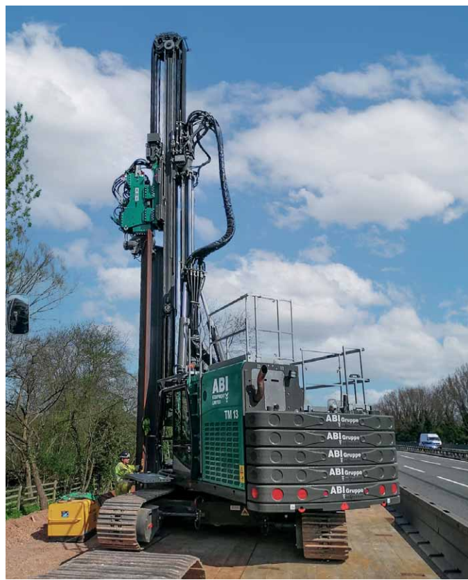
Photo: Job site of Dawson WAM Ltd - ABI MOBILRAM TM 13 with vibrator MRZV 12VV working on the smart motorway project (above)
