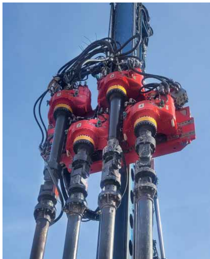
Photo: Quadmix TMBA 4-10000 with cardanic joints for easy assembly (above) Soil mixing works on a construction site in Berkeley, USA (below)
