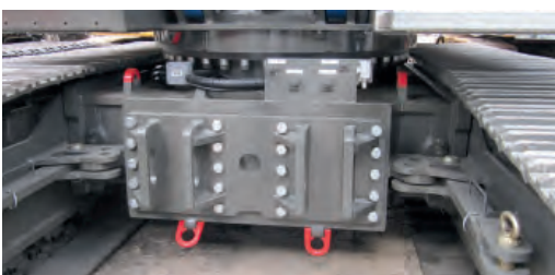
Connection for casing oscillator
