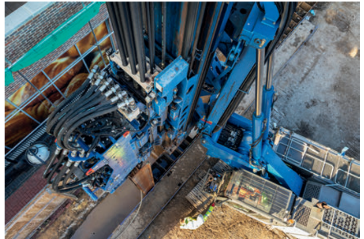
Photos: ABI MOBILRAM TM 22 with vibrator MRZV 30VV (above) and with Hydro-Press-System (below)
