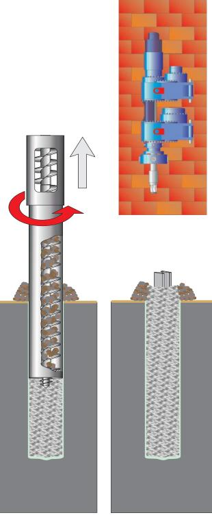
While retracting auger and casing simultaneously the concrete is being bumped in the excavation.
