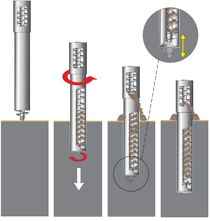
Vertical aligning of auger and casing.
