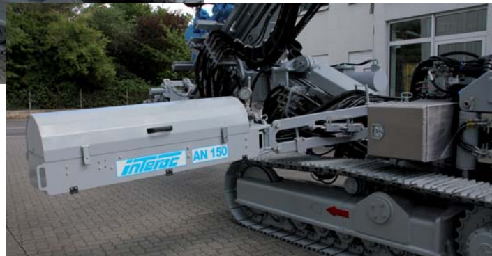
Picture: AN 150, height-adjustable control panel with open and closed vandalism protection and spacious tool box
