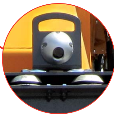
Picture: Robust camera with magnetic foot for quick removal at the counter weight of DELMAG drilling rig RH 28
