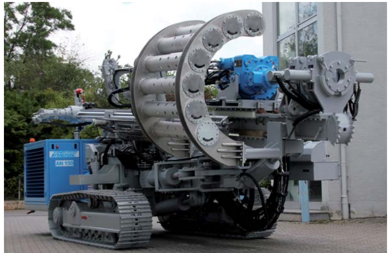
Picture: INTEROC - the unique rod changer
