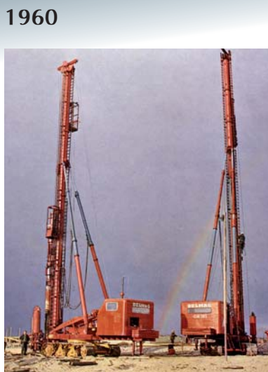
The first 18 m long lead system on crawler track GR 181 was delivered in 1964.
