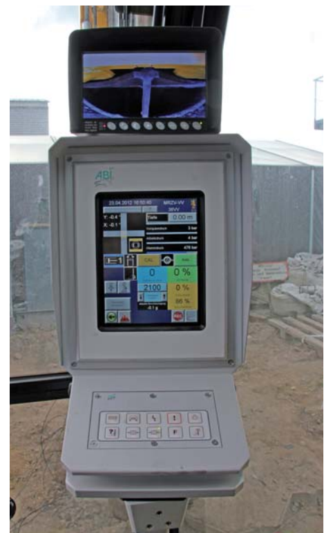
Picture: Monitor image of a clamp camera, depending on the number of installed cameras up to four views can be displayed at once.
