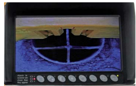
Picture: Monitor image of a clamp camera, depending on the number of installed cameras up to four views can be displayed at once.
