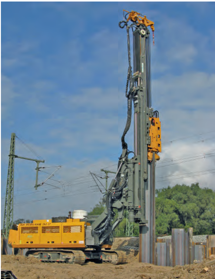
Photo: ABI MOBILRAM-System TM 17 with MRZV 28VV Vibrator
