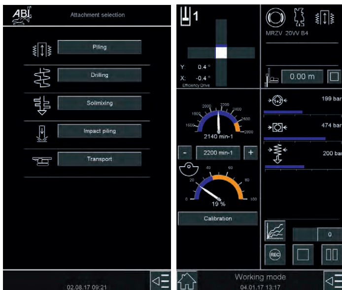
Photos: Display operation mode selector (left) and working mode for driving or extracting in manual operation mode (middle), 10 inch display in the operator's cab (right)
