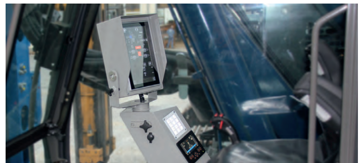
Photos: Display operation mode selector (left) and working mode for driving or extracting in manual operation mode (middle), 10 inch display in the operator's cab (right)
