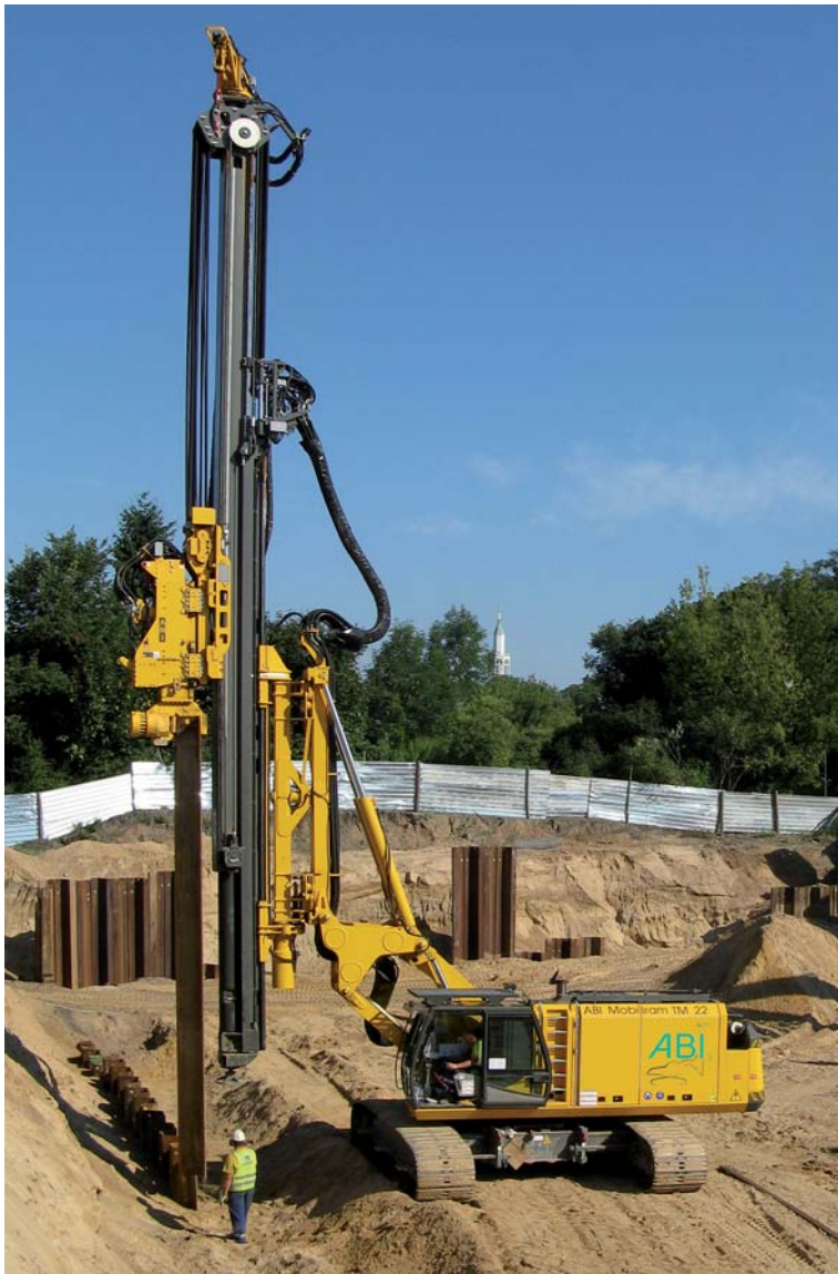
Photo left: ABI MOBILRAM-System TM 22 while pile driving
