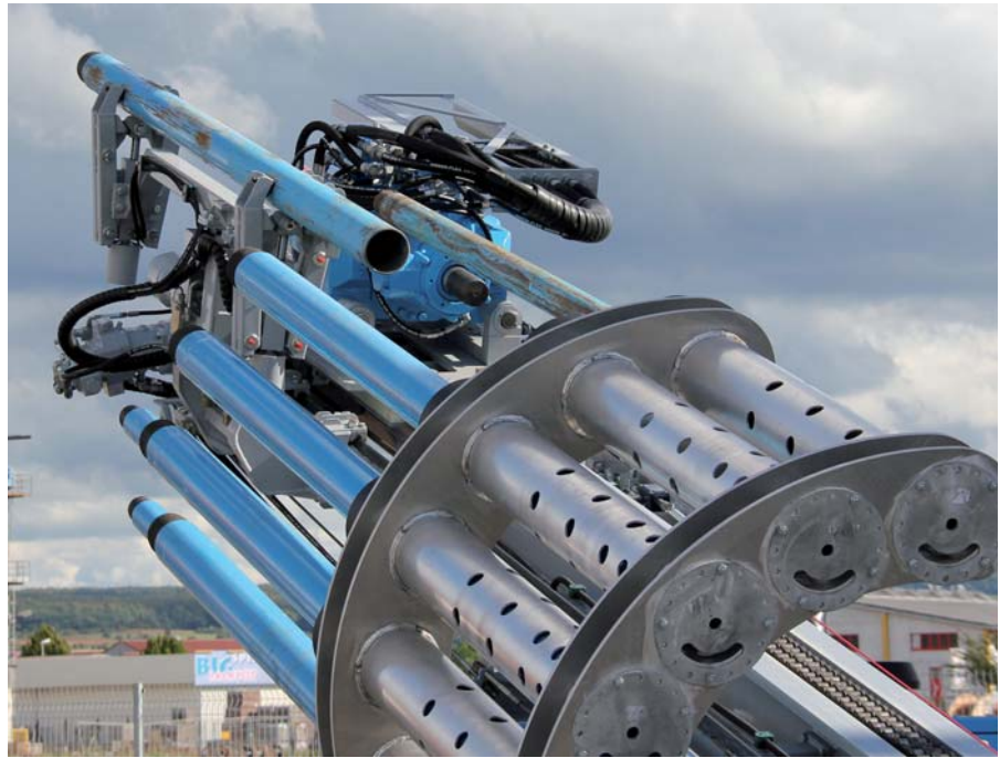
Photo: INTEROC rod changer magazin with manipulator for easier handling of double rods
