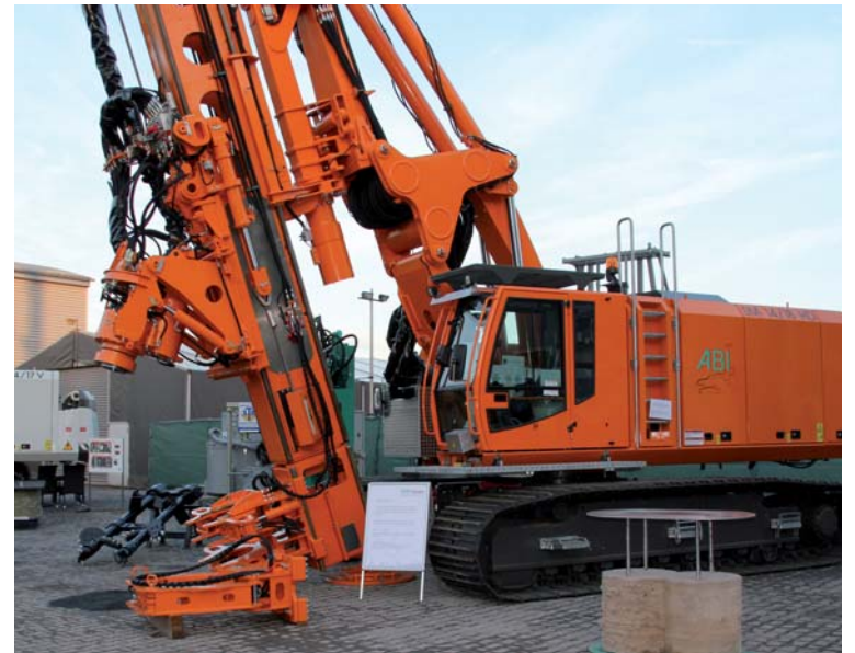
Photo: SM 14/18 HD with auger drive MDBA 5000 and clamping and breaking device
