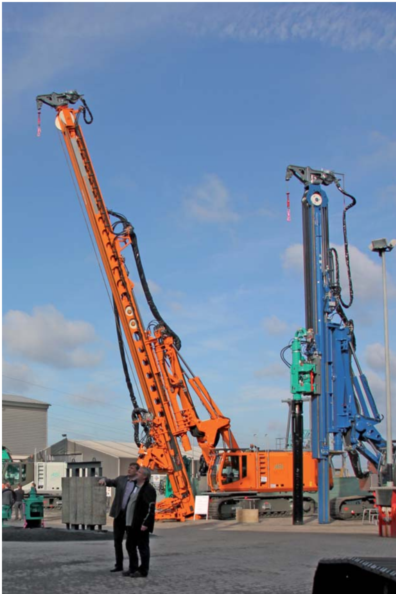
Photo: SM 14/18 HD with auger drive MDBA 5000 and clamping and breaking device
