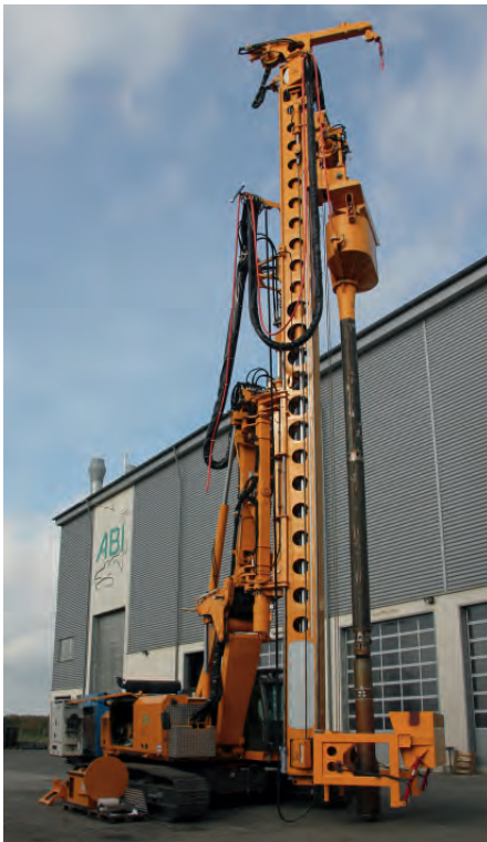
ABI MOBILRAM SM 14/18 HD equipped with vibroflot and powerfull electric generator on the back.
