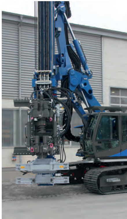
ABI MOBILRAM TM 17 with micro pile equipment, the auger drive can be moved laterally out of the drilling axis, the clamping and breaking device is used for handling the single micro pile elements.
