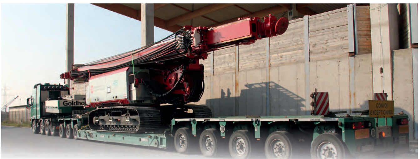
ABI MOBILRAM is driven in a transport position into a building.
