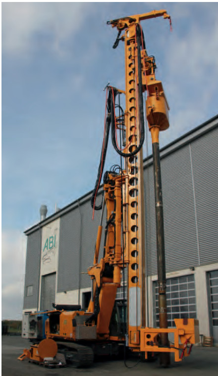
ABI MOBILRAM SM 14/18 HD equipped with vibroflot and powerful electric generator on the back.
