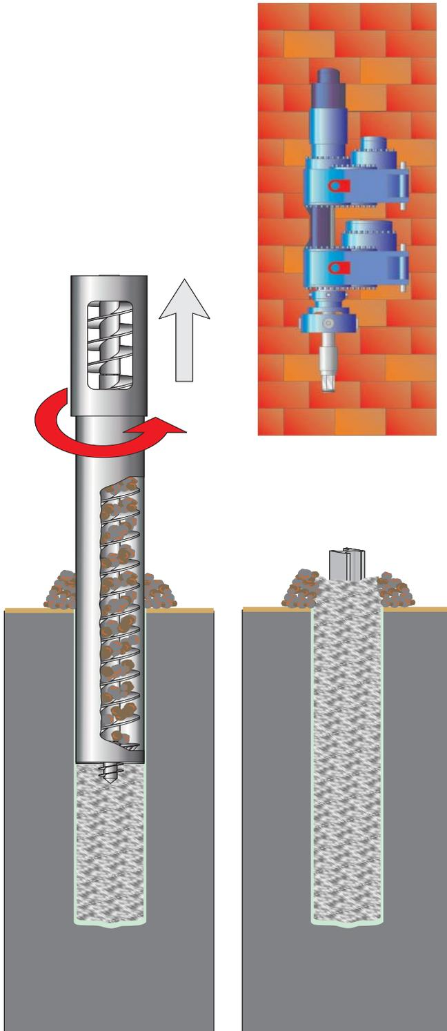
While retracting auger and casing simultaneously the concrete is being pumped in the excavation.
