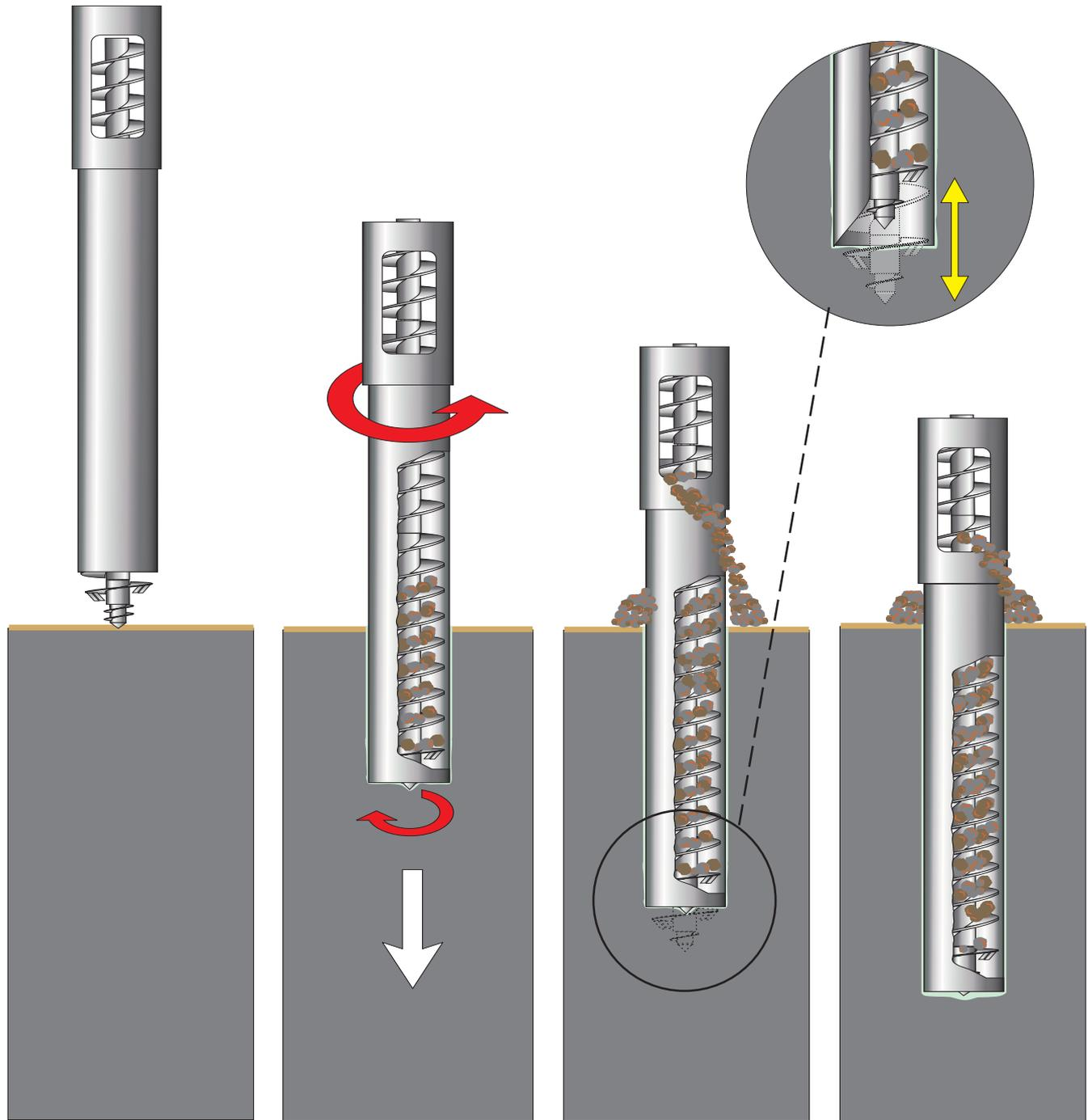
Vertical aligning of auger and casing.
