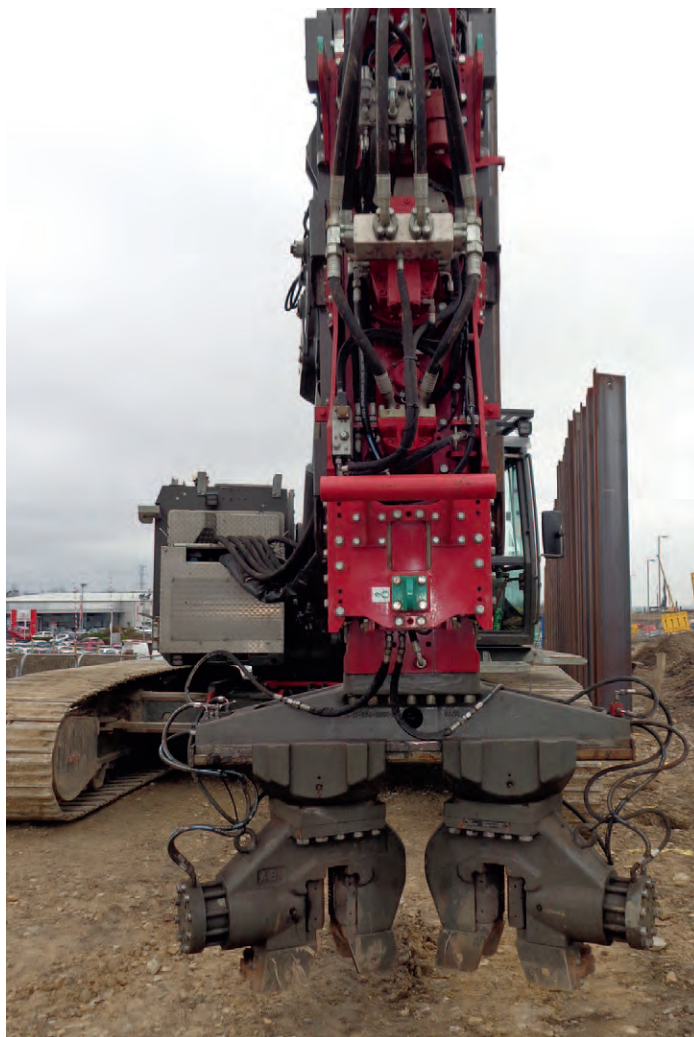
Photos: ABI combi clamp assembly MZK 1200 mounted on vibrator MRZV 30VV (above) Piling works with TM 20 in Kyleakin, Scotland (left)
