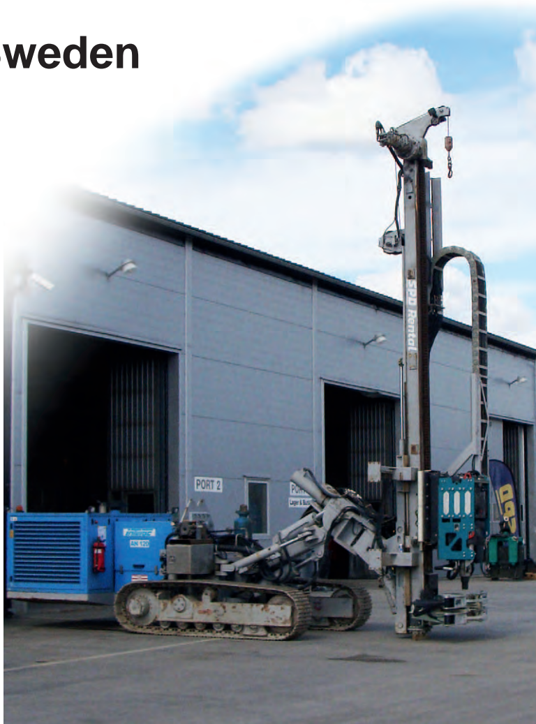
Photo: INTEROC anchor drill rig AN 120 of the SPD AB rental fleet
