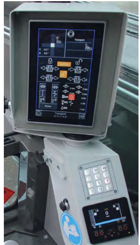
Control panel of DELMAG drill rig with keypad and big touch screen
